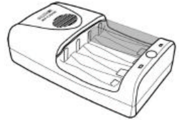
Two batteries in right bank. One hour quick charge. Suitable for AA battery > 2000mAh & AAA > 700mAh.
